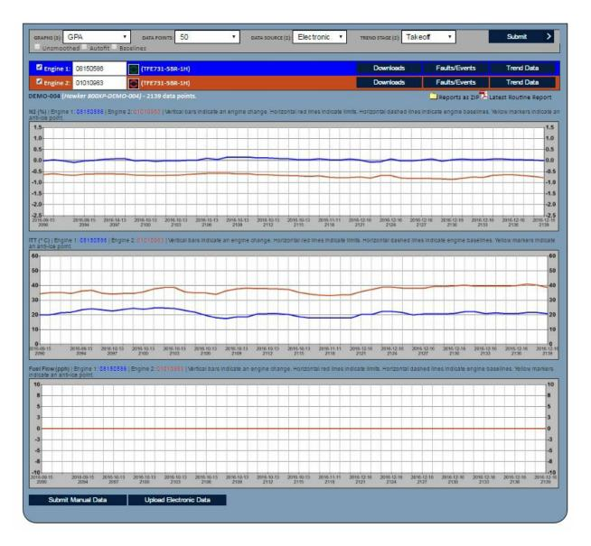
The **trend graph** shows the **engines** attached to the **current aircraft** and allows the trend stage and data source to be selected enabling the relevant trend plots to be shown.
